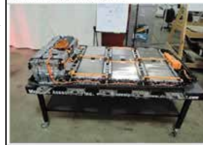
Figure 54: Chevy Bolt battery pack
